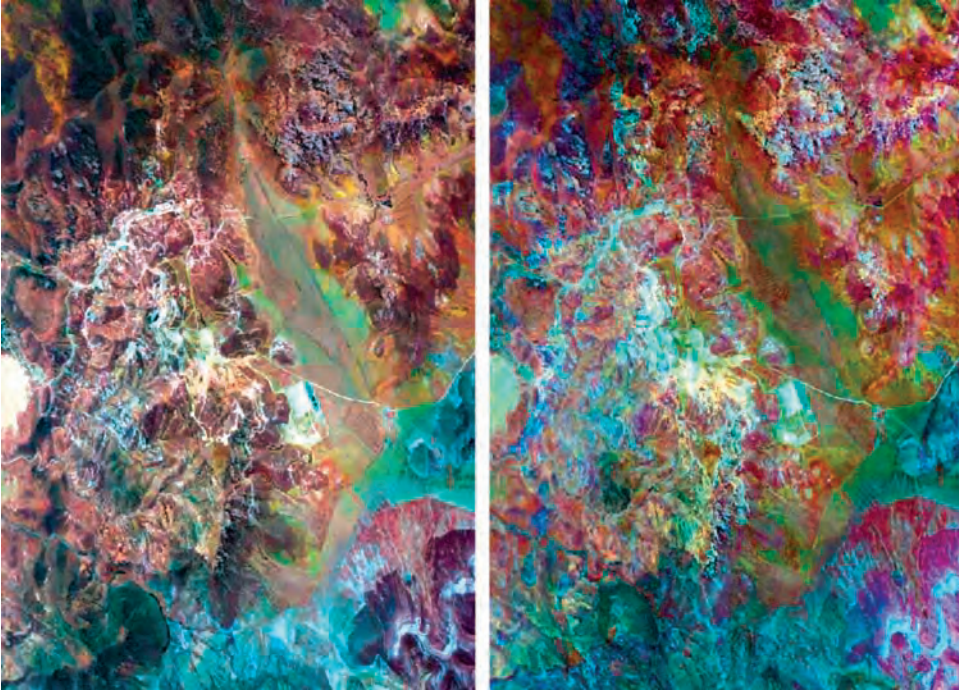
Figure 3.10 (a) The colour composite of ATM bands 9, 4 and 2 in red, green and blue; and (b) the simulated reflectance colour composite of ATM bands 9, 4 and 2
