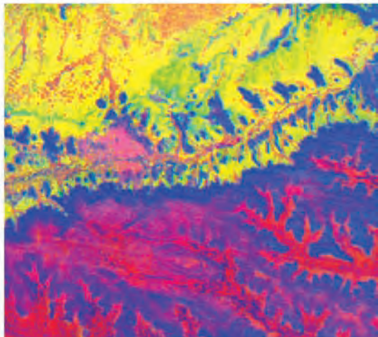
Figure 22.16 The Hargeisa area: (a) iron oxide content ( b2/b1 ); (b) silica content ( b13/b10 ); (c) carbonate index ( (b6 + b9)/(b7 + b8) ); and (d) ratio composite image produced by combining (a), (b) and (c) as RGB: desert quartz sands appearing yellow and orange, with a contribution from high silica content (green) and iron oxides (red); crystalline gneissic basements (beneath the sands) appear in yellow (high silica); the Auradu carbonates appear in bright blue tones, some patches of green appear in valleys where carbonate and silica signatures are mixed. The upper surface of the Auradu limestone plateau, and the valleys cut into it, appear red suggesting it has a strong iron oxide content, perhaps produced by a surface coating or ferricrete. Field of view is 33 km in width
