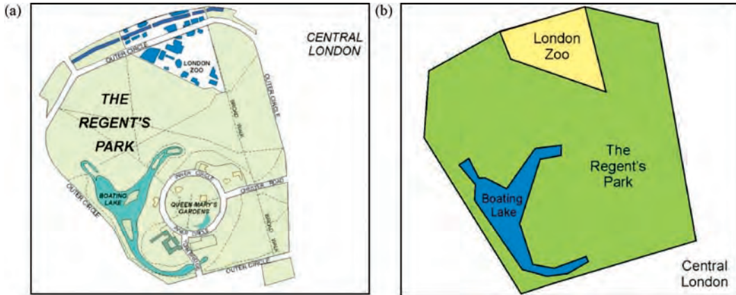
Figure 12.7 (a) A topographic map showing the Regent's Park area in London; and (b) a topological map showing the locations of London Zoo and the Boating Lake which lie inside Regent's Park in London
